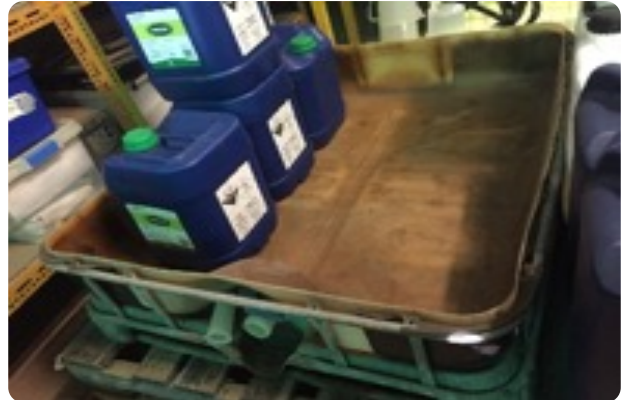
Example: Cut down shuttle used as a portable bund (for Class 8 Corrosive)
