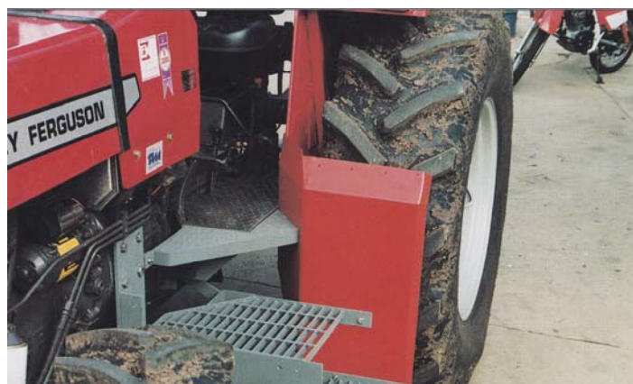
Upper and lower section of extension fitted to mudguard
